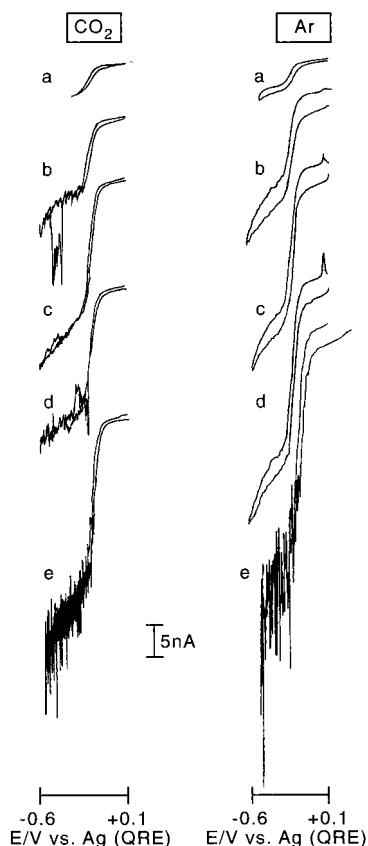
Figure 3. Cyclic voltammograms for the reduction of 1 mM \text{Ru}(\text{NH}_3)_6\text{Cl}_3 in 0.1 M KCl aqueous solution obtained at a 25 \mu\text{m} diameter Pt microdisk electrode at 20 ^\circ\text{C} . Scan rate, 50 mV/s. Conditions: \text{CO}_2 , 8.3 bar, (a) silent, (b) 1%, (c) 10%, (d) 20%, and (e) 30% relative ultrasound power; Ar, 8.9 bar, (a) silent, (b) 10%, (c) 30%, (d) 50%, and (e) 60% relative ultrasound power.
